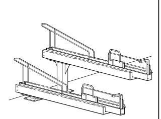
Fix one rack to the top of each mounted pole
