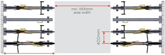
To **comply** with AS2890.3 (2015) minimum 400mm spacing between bikes,
