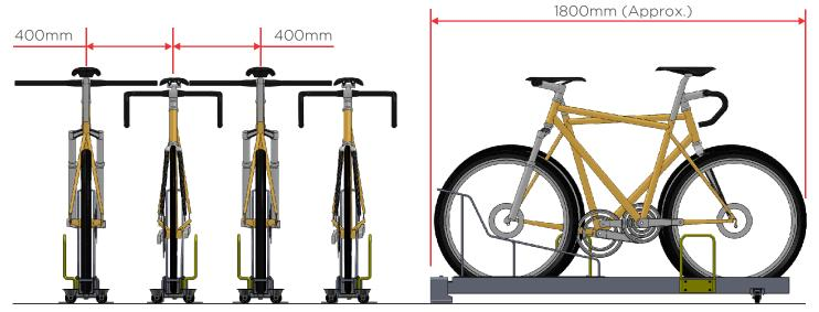
To **comply** with AS2890.3 (2015) minimum 400mm spacing between posts centres and to edge of walls or other obstructions
