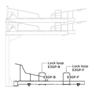
Choose either the E3GP-B or E3GP-F E3GP-B - Back wheel in first E3GP-F - Front wheel in first
